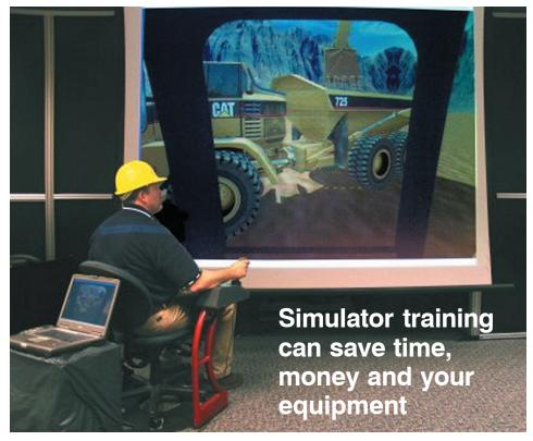
experience in the cab of a real machine. Working independently or with an instructor, the trainee can participate in a series of 12 gradually more difficult scenarios. These teach basic operations of the excavator, from how to move the bucket and position the boom right up to trenching and safely loading a truck.
